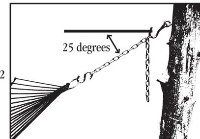
of the chain as illustrated in Figure 2 is at least 25 degrees from horizontal. Hanging your hammock more tightly than this greatly increases the load to the hardware and supports.
